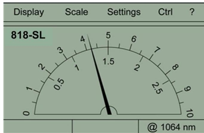
Fig. 2-7 Digital Needle Display
